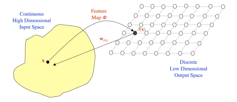
Each point I in the output space maps to a corresponding point w(I) in the input space.
