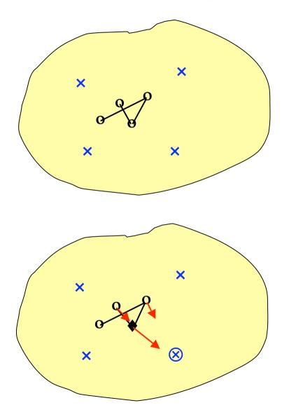
Suppose we have four data points (crosses) in our continuous 2D input space, and want to map this onto four points in a discrete 1D output space. The output nodes map to points in the input space (circles). Random initial weights start the circles at random positions in the centre of the input space.
