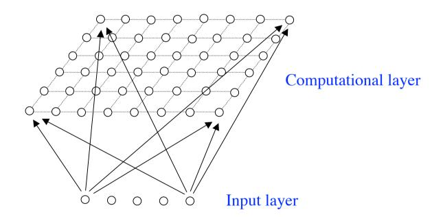
Clearly, a one dimensional map will operate in the same way but just have a single row (or a single column) in the computational layer.
