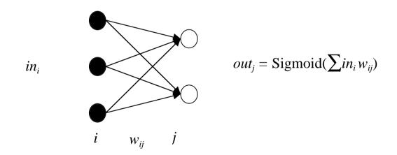
The standard procedure is to define an output error measure (such as the sum squared difference between the actual network outputs and the target outputs), and use *gradient descent* weight updates to reduce that error. The details are complex, but such an approach can learn from noisy training data and generalise well to new inputs.
