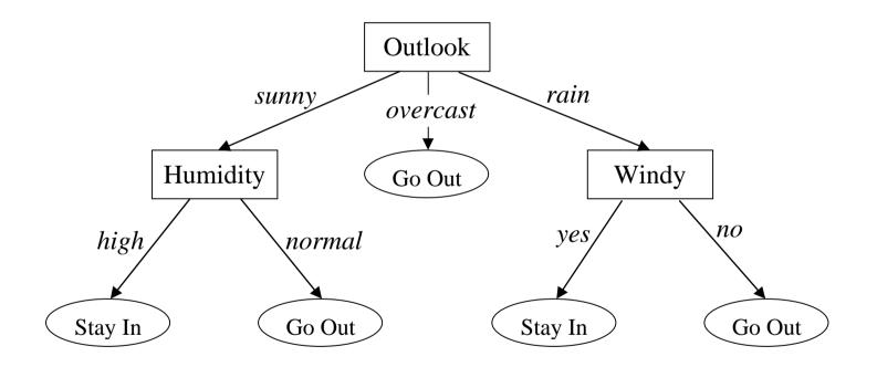
Intermediate nodes represent choice points, or tests upon attributes of the data, which serve to further sub-divide the data at that node.
